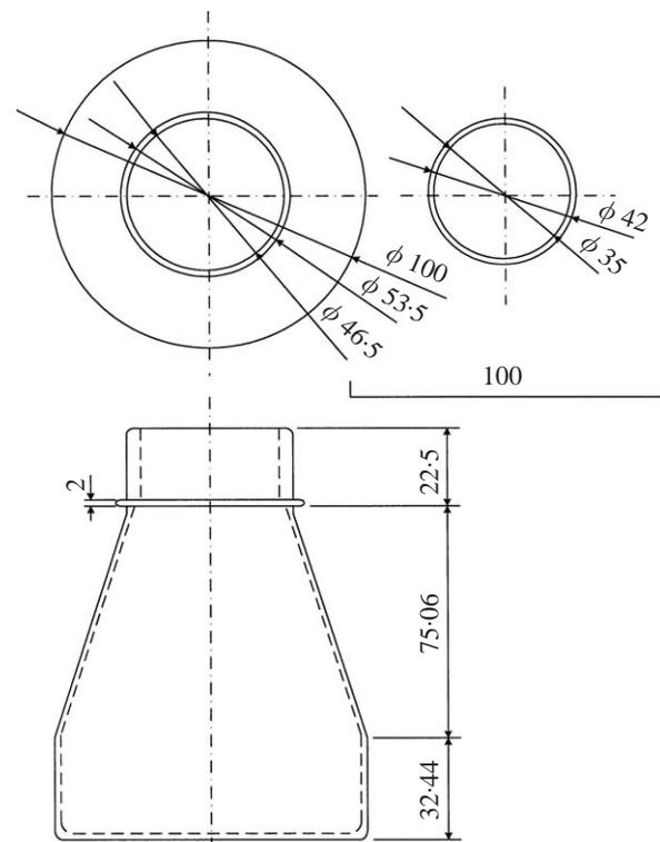
Fig. 1. Schematic diagram and size of conical plastic flask; all dimensions in mm
