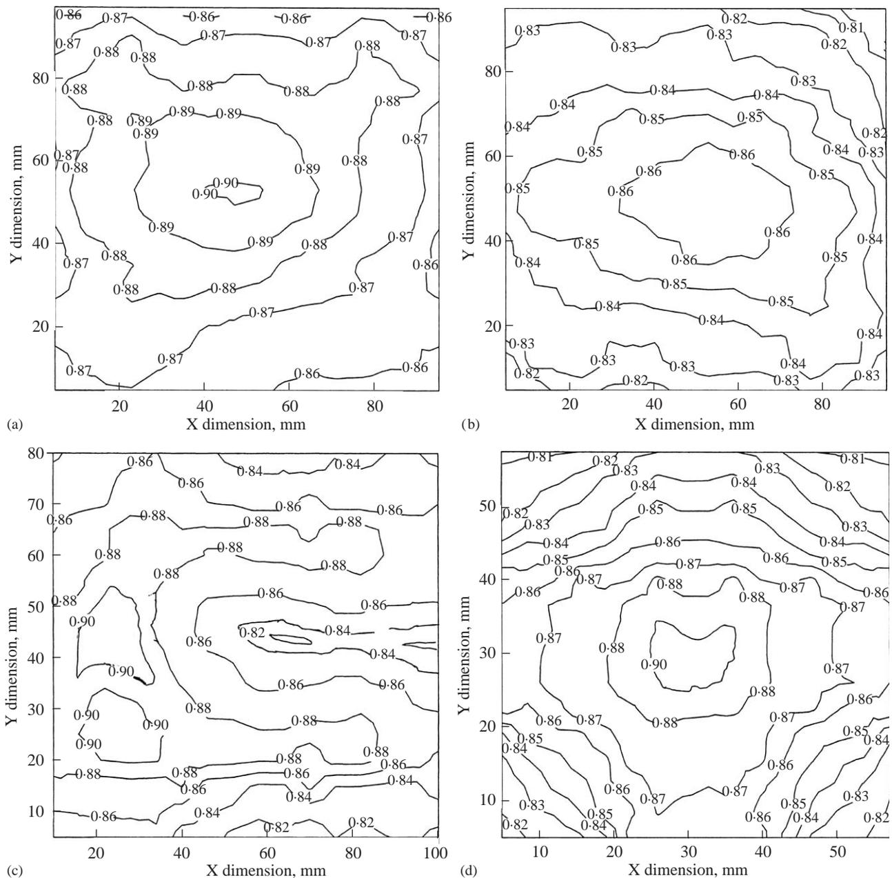
Fig. 7. The contour curves of flux density transmittance of (a) conical glass flask, (b) conical plastic flask, (c) Japanese irregular box, (d) GA-7 vessel, (e) round vessel, (f) square box, and (g) rectangular box
