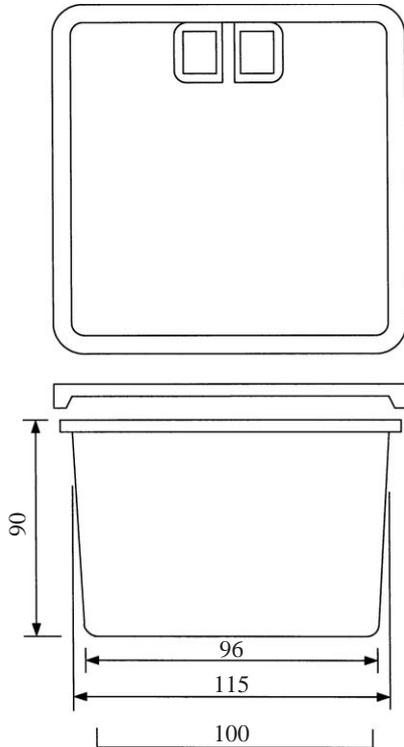
Fig. 4. Schematic diagram and size of square vessel; all dimensions in mm
