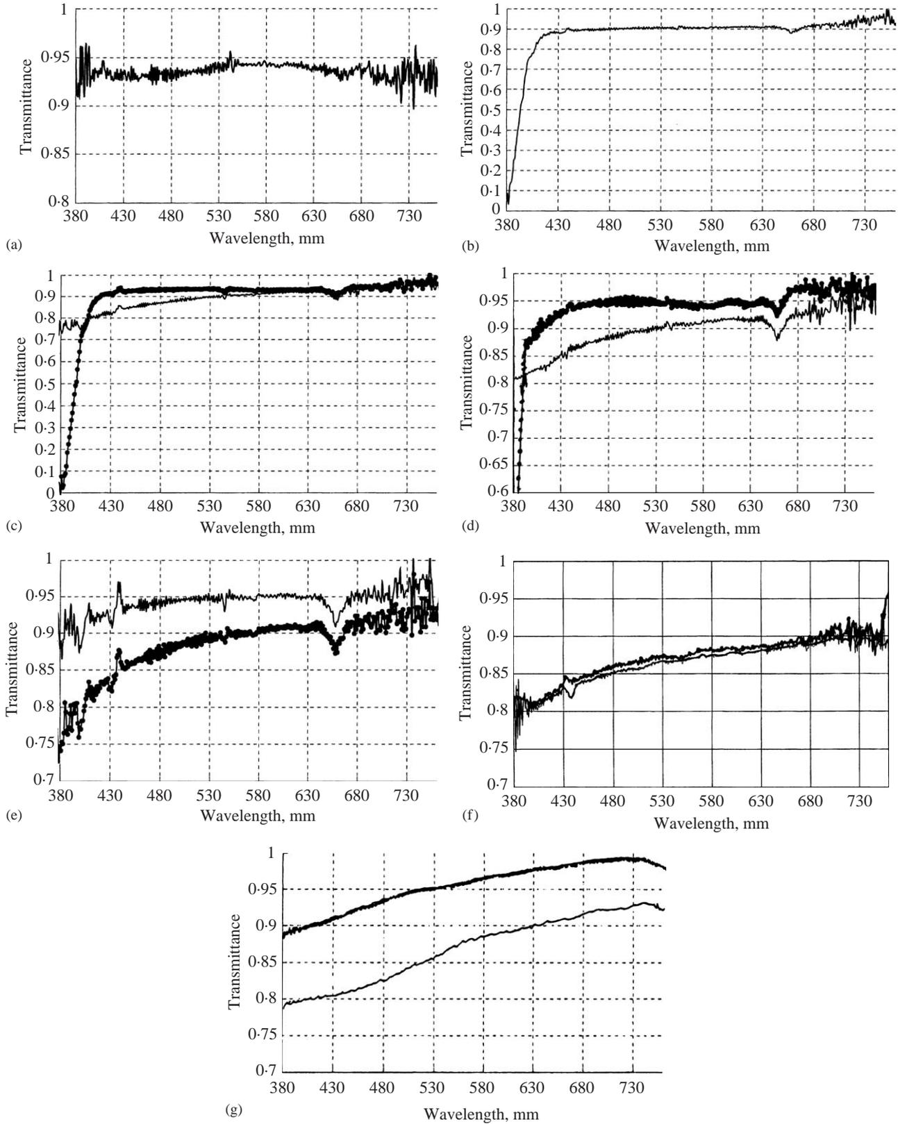
Fig. 8. The distribution of spectral transmittance of (a) conical glass flask, (b) conical plastic flask, (c) Japanese irregular box, (d) GA-7 vessel, (e) round vessel, (f) square box, and (g) rectangular box: \_\_\_\_\_, wall; \_\_\_\_\_, lid
