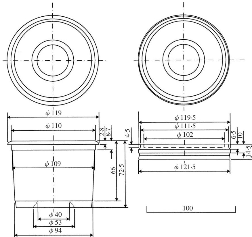
Fig. 3. Schematic diagram and size of round vessel; all dimensions in mm
