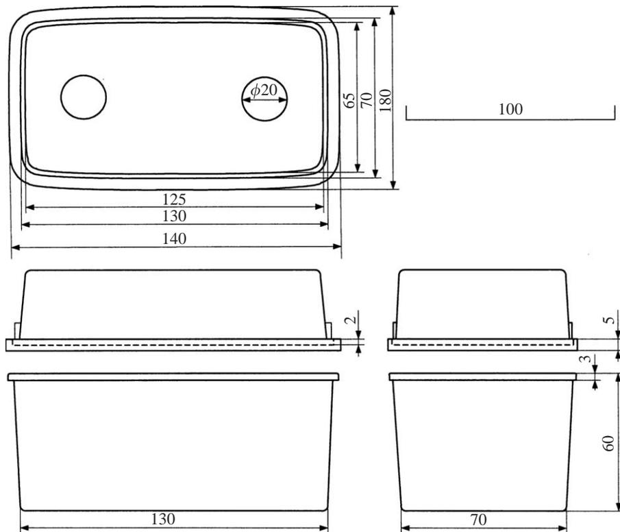
Fig. 5. Schematic diagram and size of rectangle vessel; all dimensions in mm
