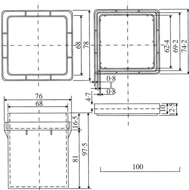
Fig. 2. Schematic diagram and size of GA-7 vessel; all dimensions in mm
