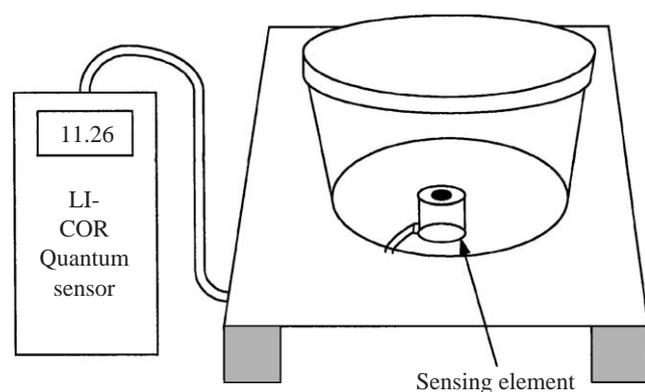
*Fig. 6. Measurement of the internal transmittance of round vessel*
